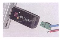
Strip off approximately 5 mm of the insulation on the external equipment's control wires. Fasten the stripped wires to the screw terminal on the connector plug. Be careful to insert the stripped wire ends completely into the screw terminal and to fasten the screws accurately! Insert the
